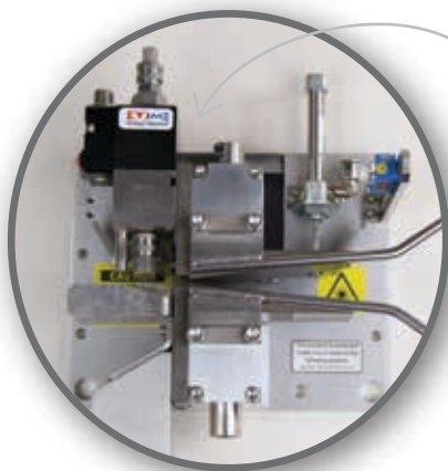
900 Series Cold Glue Valve on a BoardRunner® glue station
