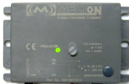
Green Light → Full; Output not activated
