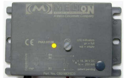
Red-Yellow blinking light → Full; Output activated, delay at disconnect
