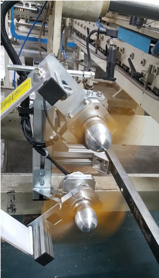
These pictures show the electric trim removal installed on a flexo-folder machine.
