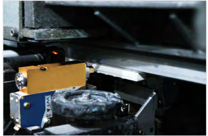
In side-seam gluing processes, applicators may be mounted to apply the adhesive to the book block (as shown) or to the cover feeder.
