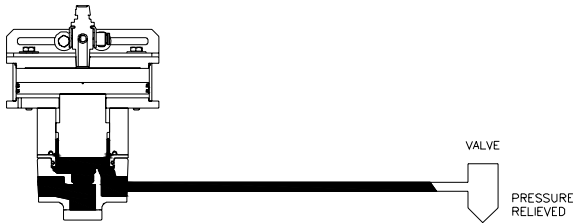
No Pressure (Machine Stopped)
