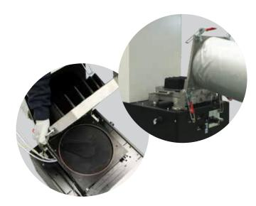
Its tiltable tank and removable melting grid facilitate maintenance and cleaning operations, which may be carried out faster and safer.
